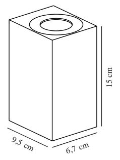
Voltage (V): 230 Volt IP degree: IP44 Class (Class 1, Class 2, Class 3): Class 1 (Earth contact) Socket type: LED – Nonreplaceable light source Parallel connection: True
