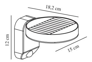
IP degree: IP44 Class (Class 1, Class 2, Class 3): Class 3 (Low voltage) Socket type: Solar LED – Nonreplaceable light source
