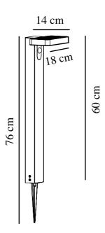
IP degree: IP44 Class (Class 1, Class 2, Class 3): Class 3 (Low voltage) Socket type: Solar LED - Nonreplaceable light source
