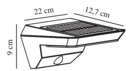
IP degree: IP44 Class (Class 1, Class 2, Class 3): Class 3 (Low voltage) Socket type: Solar LED – Nonreplaceable light source
