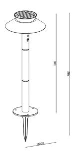
Voltage (V): 3,7 Volt IP degree: IP44 Class (Class 1, Class 2, Class 3): Class 3 (Low voltage) Socket type: Solar LED – Nonreplaceable light source
