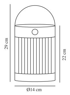
Voltage (V): 5 Volt IP degree: IP44 Class (Class 1, Class 2, Class 3): Class 3 (Low voltage) Socket type: Solar LED – Nonreplaceable light source Switch placement: On the fixture Parallel connection: False
