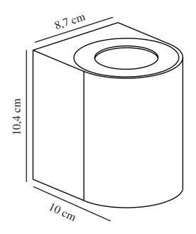
Voltage (V): 230 Volt IP degree: IP44 Class (Class 1, Class 2, Class 3): Class 1 (Earth contact) Socket type: LED – Nonreplaceable light source Dimmerable - Hidden: False Parallel connection: True
