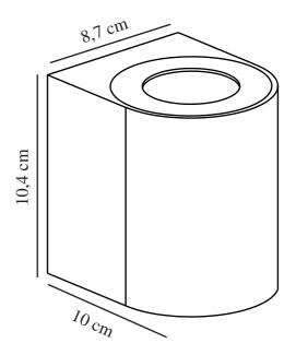
IP degree: IP44 Class (Class 1, Class 2, Class 3): Class 1 (Earth contact)
