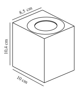
Voltage (V): 230 Volt IP degree: IP44 Class (Class 1, Class 2, Class 3): Class 1 (Earth contact) Socket type: LED – Nonreplaceable light source Dimmerable - Hidden: False Parallel connection: True
