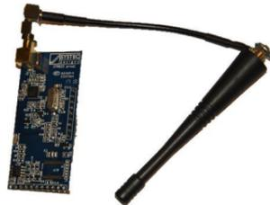
The Zehnder RF-PCB enables the CCRFZ (655 000 755) controller to be used with the ventilation system without the need for the ComfoSense C67.
