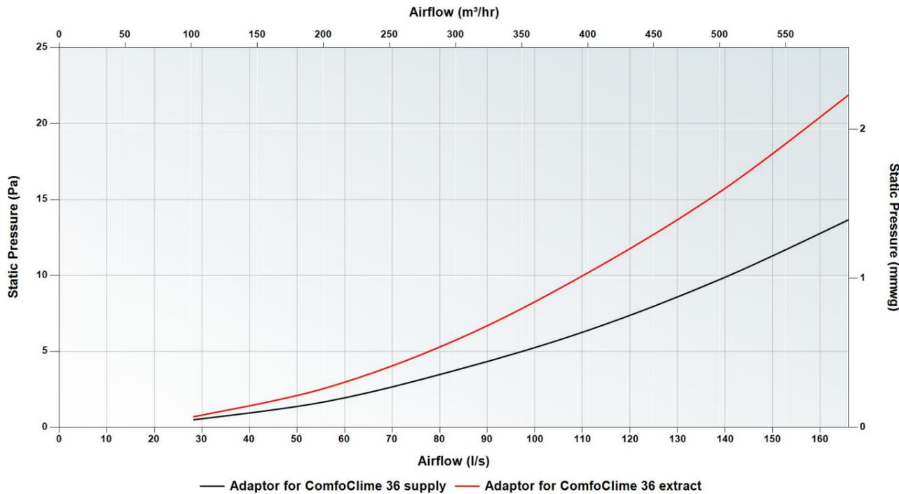
**Steel ducting ø 215 mm to ø 200 mm reducer for ComfoClima 36, galvanised**
