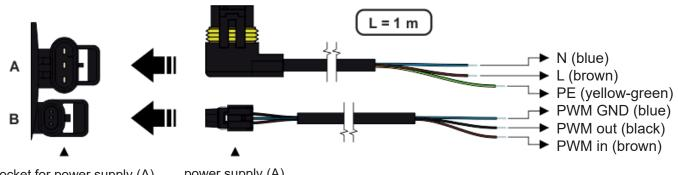
socket for power supply (A) and signal transmission (B)
